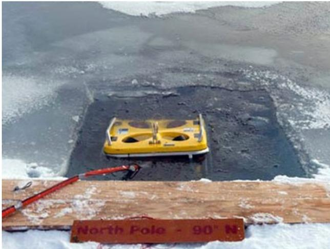
The ROV is operated directly from the sea ice while the ship anchors on an ice floe for several hours. The vehicle is launched through melt pond holes, which are present on the ice during this season, and controlled from a tent on the ice. The work directly from the sea ice reduces the effects of the vessel on the measurements and enables direct sampling of the ice along the transects.
