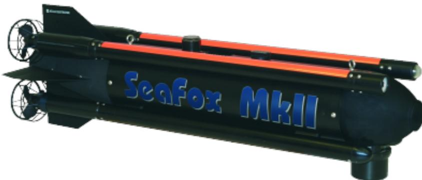
ATLAS is constantly improving the SeaFox suite. The new SeaFox MkIII is being fitted with a novel type of fuse that will allow safe on-board recovery of the SeaFox C if it is not used after deployment. Until now, once a SeaFox was launched, it always had to be detonated after a certain time window had elapsed. A new Mobile Control Unit will also be offered.
