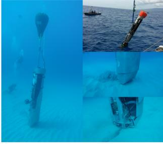
Makai Ocean Engineering and the University of Hawaii (UH) have jointly developed a novel autonomous underwater vehicle (AUV) that can effectively deploy seafloor sensing equipment by combining features of a free-swimming AUV and those of a bottom crawling vehicle.
