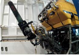
Using a remotely operated underwater vehicle with an installed saw, researchers have acquired geological samples from the Jan Mayen Ridge this summer.
