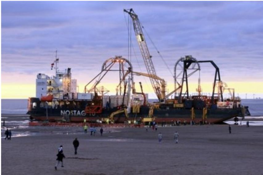
Local people flock to see the *Nostag 10* at Barkby Beach as it connects the cables that will travel out to sea to Ireland. As it makes its way across the sea, the cable will be carefully lowered into the water and laid in a narrow trench which will be opened and closed by a remote controlled vehicle operating on the sea bed. The cable laying work is expected to take approximately eight months to complete.
