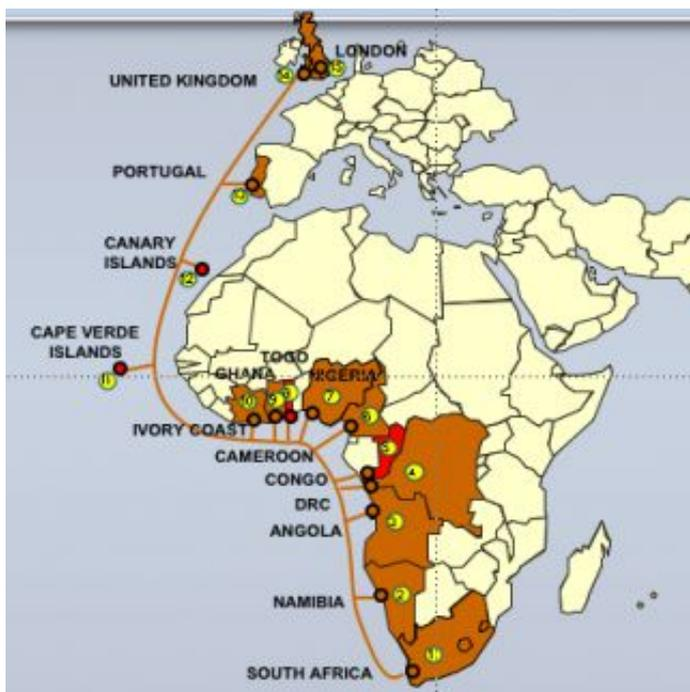
The WACS submarine cable is an ultra high capacity fiber optic submarine cable system which links Southern Africa and Europe, spanning the west coast of Africa and terminating in London, United Kingdom. This \$650 million cable
