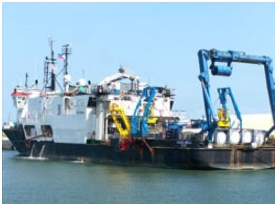
*Allied Shield* uses thrusters on its sides to keep it in place (dynamic positioning) directly above *Solar 1*. A global positioning satellite also continuously checks its position relative to the sunken vessel.
